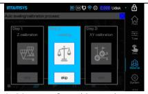
1. Measure 3 position points on the buildplate with the help of the leveling sensor on the nozzle, determine the relative position of the buildplate and the XY motion plane, and perform Z-direction compensation during the printing process. Click the **Leveling** icon, and a prompt box will pop up to remind you to clean the buildplate, chamber and nozzles to prevent interference with the leveling operation.
