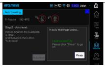
4. After the three-point automatic leveling is successful, click the **Finish** button, and the buildplate will move downward and upward to the origin of Z axis.
