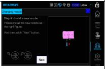
New Nozzle Installation: Follow the prompts to replace the nozzle and reinstall the fan cover and printhead cover. Note: After replacing the nozzle, A recalibration and leveling operation is necessary
