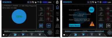
6. When the progress shows 100%, the printing is completed, after the temperature drops to a safe temperature, you can click 🛄 to open the door and take out the printed model.
