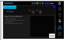
6. Follow the on-screen instructions and click the **Finish** button to end the calibration. After the operation is over, take out the digital indicator and close it.
