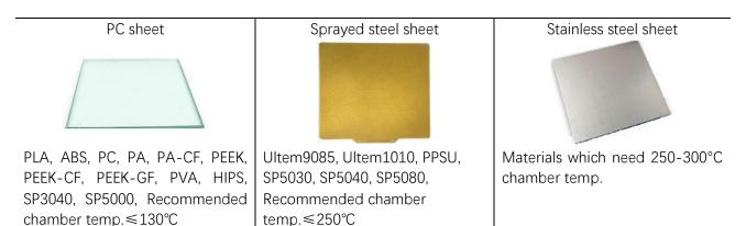
Note: The sprayed steel sheet and stainless steel sheet need to be heated in the chamber before vacuum adsorption, to ensure that the temperature of the buildplate is higher than 160 °C, and the vacuum adsorption can be performed normally after the stress is released.
