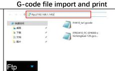
1-2. Ftp (network): enter the IP address of the printer in the address bar of the window folder on the computer, and transmit the G-code file to the printer through the network.
