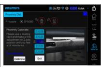
3. Use a leveling card(0.2mm thickness) and click "Z<sup>↑</sup>0.05" or "Z<sup>↓</sup>0.05" to make preliminary adjustments, and click "Z<sup>↑</sup>0.01" or "Z<sup>↓</sup>0.01" to make fine adjustments, the distance between the nozzle and the buildsheet just put in the card. Take out the card and click the Calibrate icon to complete the trigger distance calibration, click the Exit button to complete the general calibration.
