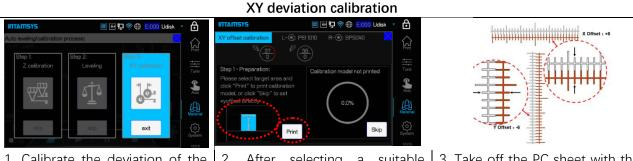
1. Calibrate the deviation of the left and right nozzles in the X and Y directions, the deviation value is obtained by actually printing the calibration model. Click **XY Calibration** to enter the subpage, follow the prompts.
