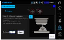
5. The buildplate will first descend and switch to the right nozzle, and then rise to make the right nozzle contact the digital indicator. The value displayed on the digital indicator is the Z deviation value of the left and right nozzles. Enter it into the dialog box on the screen and save it. You can click the Recalibrate button on the screen to repeat the calibration steps. If the two calibration results are consistent, the calibration value is reliable.
