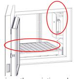
Cleaning the printing chamber: The materials left on the bottom plate or dropped during the printing process need to be cleaned up in time to avoid affecting the next printing. Use a vacuum cleaner and a removal tool to clean the waste and residue at the bottom of the chamber, side walls, etc.. Wipe with a cleaning cloth and alcohol if necessary..
